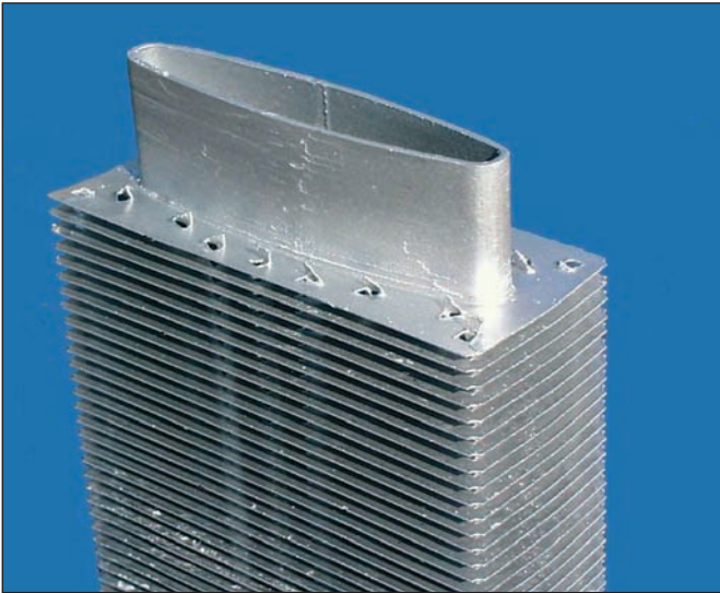
Figure 8: Matimba ACC heat exchanger tube. The tubes are 9.5 m (31.7 ft) long. The rectangular fin dimensions are 120 and 50 mm (4.7 and 1.96 in).
