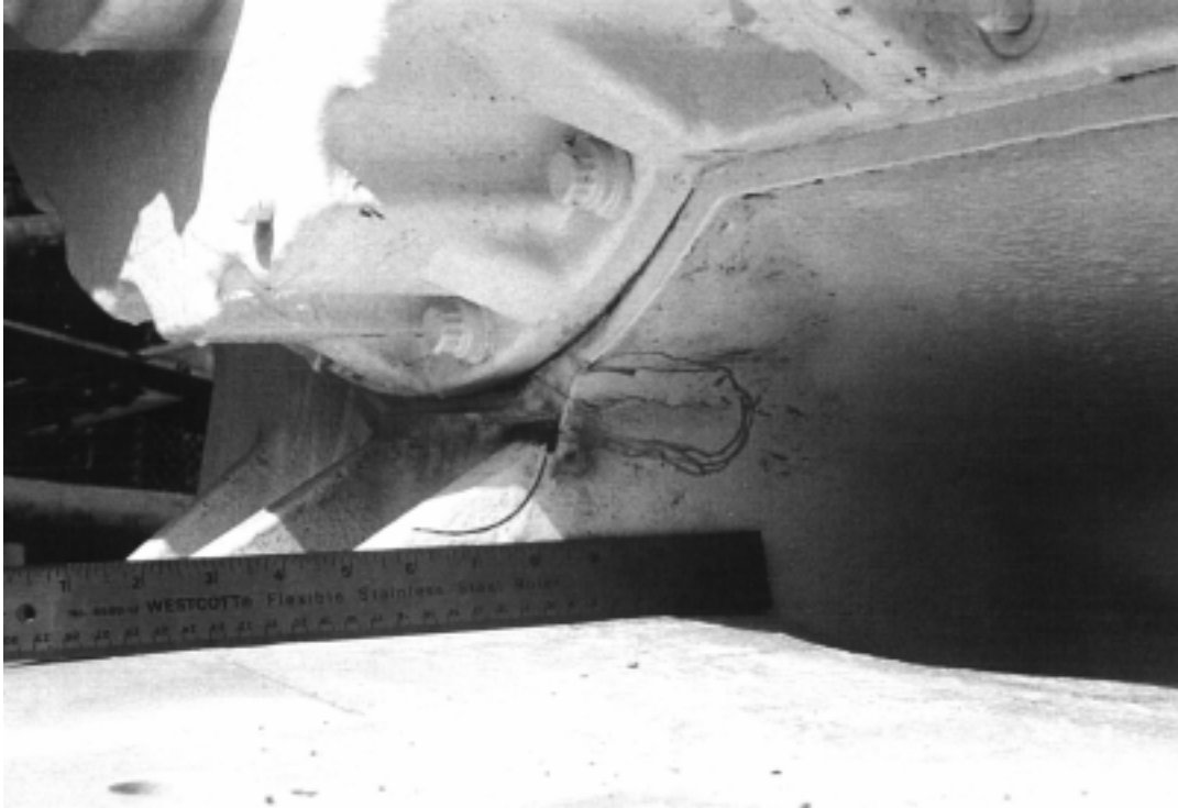
Figure 1. Photograph of Severely Cracked Transmission Housing
