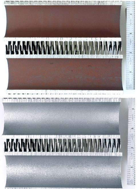
Deposit loading coupons before and after cleaning from tube with light deposits.
