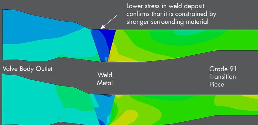
FEA output showing spatial distributions of creep-redistributed von Mises equivalent stress TOP and maximum principal stress BOTTOM in the modeled weldment.
