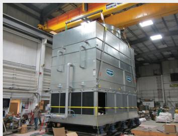
Cooling Tower Shake Table Test
