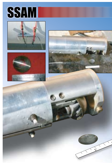
Down-bore miniature sampling tool
