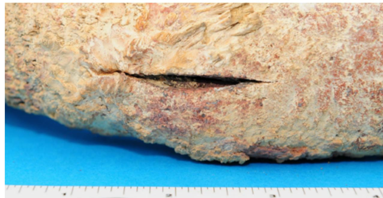
Thick-edged longitudinal rupture in tube section
