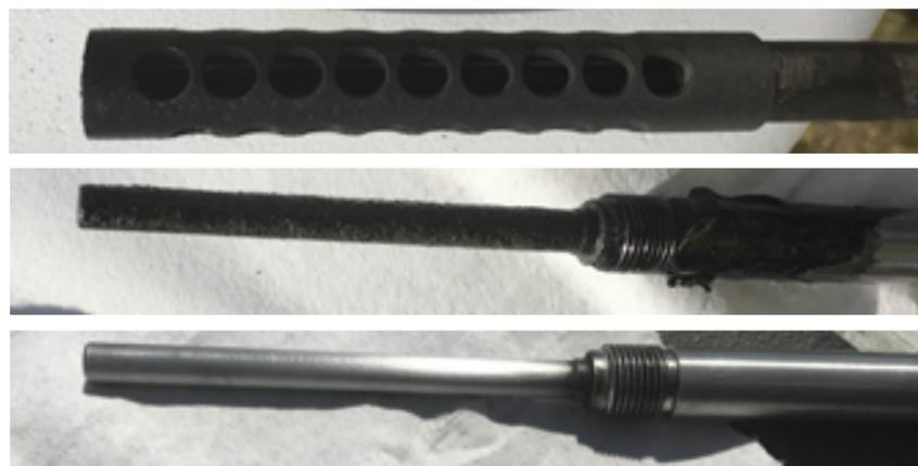
FIGURE 4. TOP ER Probe as removed MIDDLE ER Probe with Velocity shield removed BOTTOM ER Probe after samples collected & cleaning
