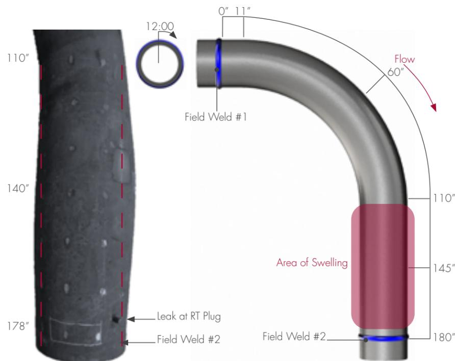
FIGURE 1. Swelled P91 Main Steam Piping
