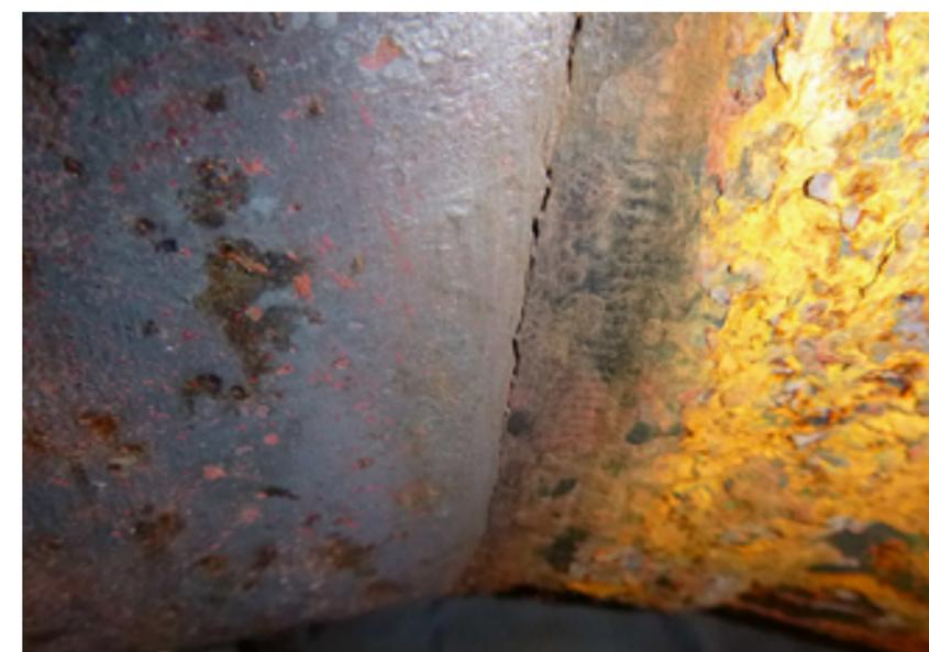
in strength to both the valve body material and the Grade 91 piping. The course of action taken was to perform local stress analysis and remaining life estimates for the downstream (outlet) connections of the valves to assess likelihood of future damage and establish an appropriate re-inspection interval. Detailed metallurgical analysis was also performed on a ring (entire
