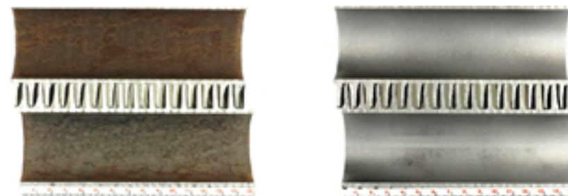
FIGURE 1. Deposit loading coupons before and after cleaning from tube with heavy deposits.
