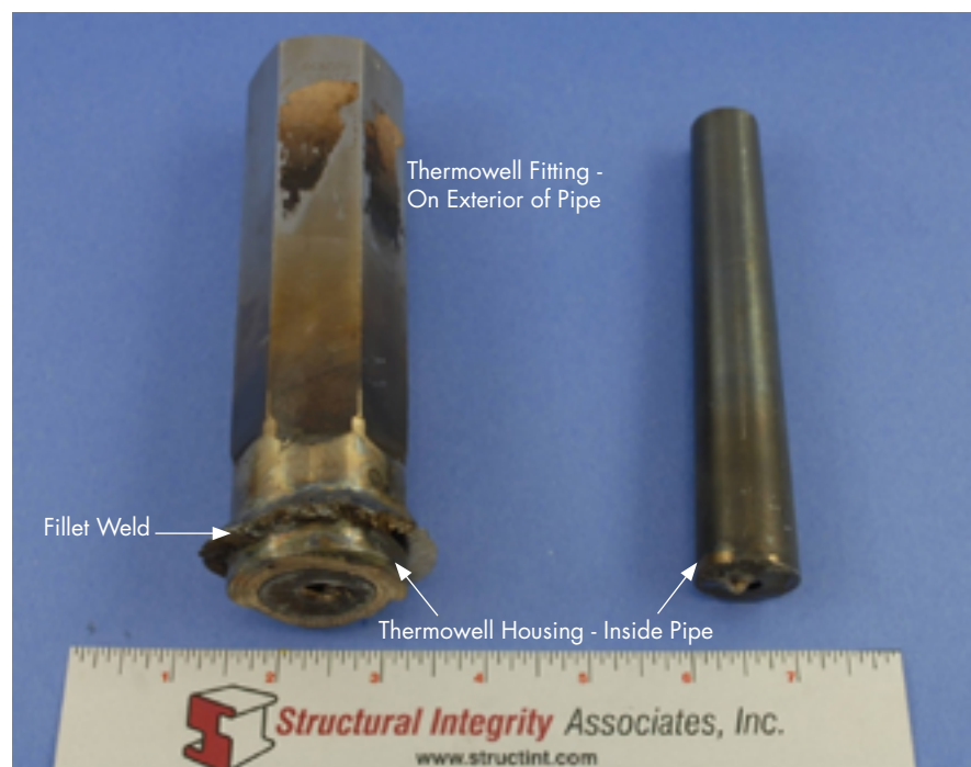
FIGURE 1. The fractured thermowell sections shown in the as-received condition. The mating fracture surfaces are facing down on each section.
