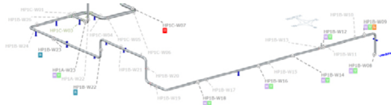
FIGURE 4 Example PlantTrack Screen Showing Welds to Be Inspected
