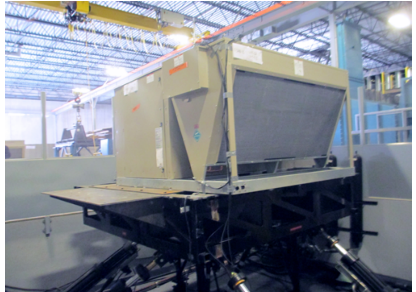
Air Conditioning Product Undergoing Shake Table Testing
