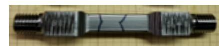
FIGURE 8. Typical cross-weld creep-rupture test specimen after final machining. The approximate locations of the weld fusion lines are marked in the gauge section.
