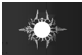
FIGURE 13. Representative Max Principal Concrete Strain Around Equipment Hatch; Peak SIT Test Pressure; 60 Year Losses
