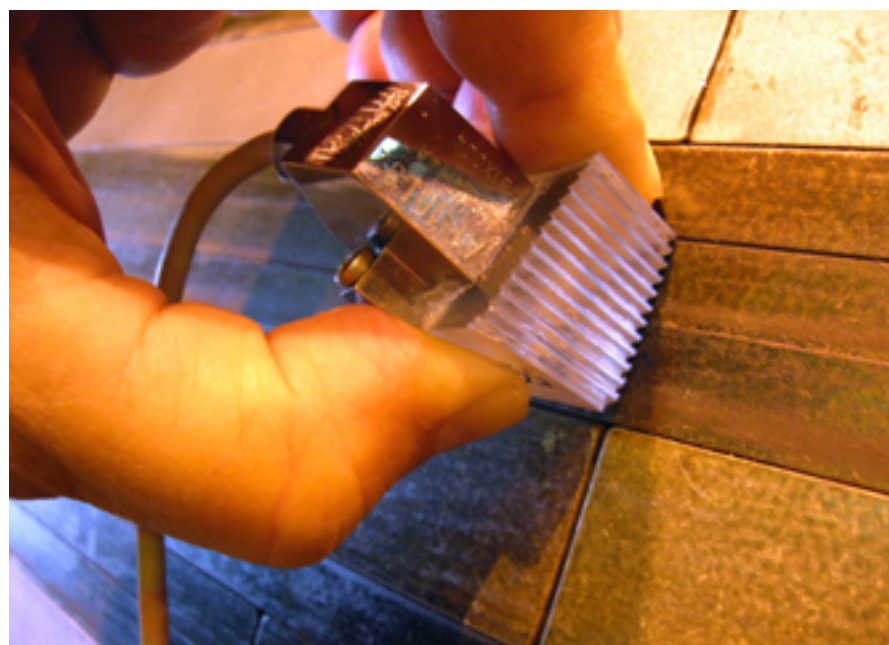
FIGURE 7. Manual LPA inspection of crush surface at the wedge butt joints with wedges installed.
