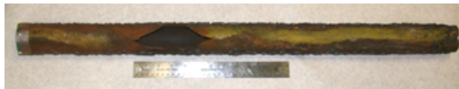
Thin edged rupture due to fire side corrosion
