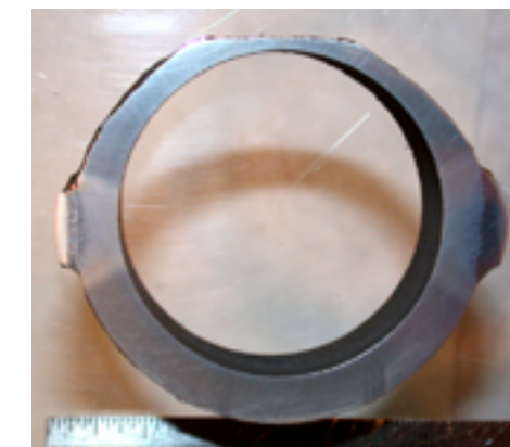
Ring section through area adjacent to rupture showing external wastage around hot side of tube with most severe wastage at crown of tube
