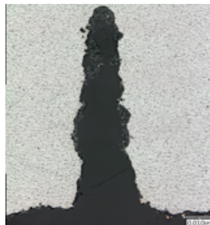
FIGURE 9. Higher magnification of the deepest location from Sample B. The copper is more clearly observed.
