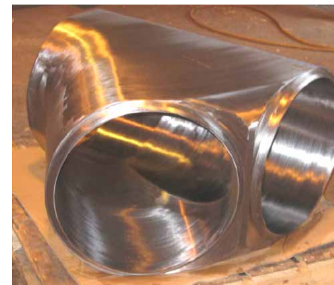
FIGURE 8. Example of a fully contoured, uniform forging that can eliminate these problematic saddle weld joints.
