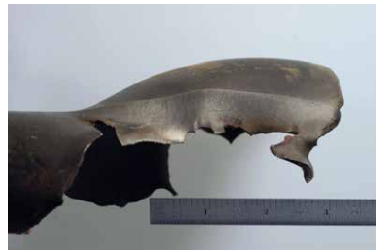
FIGURE 1. View of a ruptured tube. The flat spots associated with severe wall loss are characteristic of SBE.
