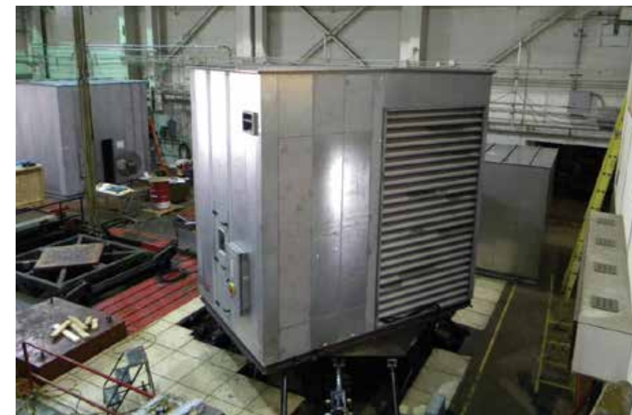
FIGURE 2. Modular air handling unit undergoing seismic testing
