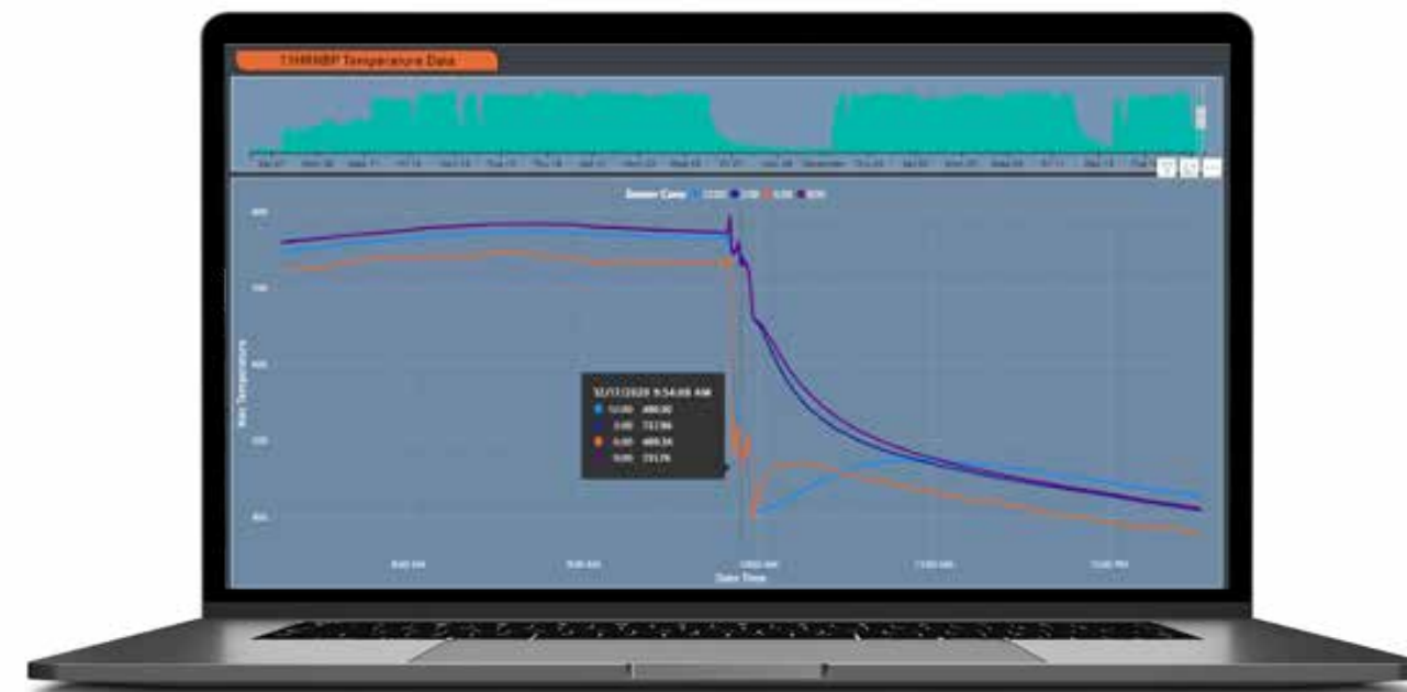
FIGURE 7. Post-outage data for the hot reheat bypass system that experienced a failure.
