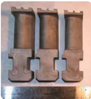
Cracked turbine blades
