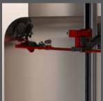
Used to deploy ultrasonic and eddy current probes on the inner surface of a vessel
