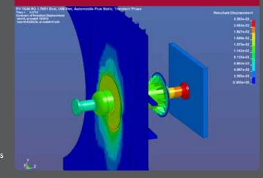
LEAK-BEFORE-BREAK EVALUATIONS | LOAD DROPS, MISSILE IMPACT, AND SHOCK 11
