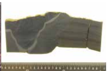
Failed downstream Weld/Elbow
