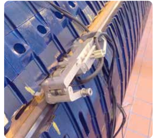
Generator rotor dovetail inspection
