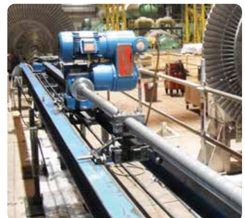
Rotor bore machining and surface conditioning
