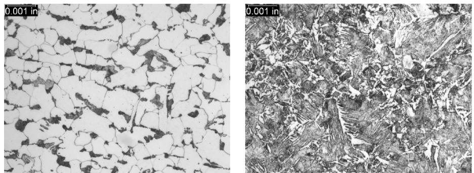
FIGURE 2. The typical microstructures from the marked sample **LEFT** and the unmarked sample **RIGHT**.
