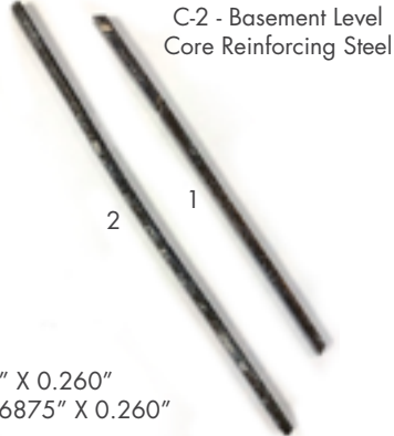
FIGURE 1. The core reinforcing steel samples in the as-received condition.
