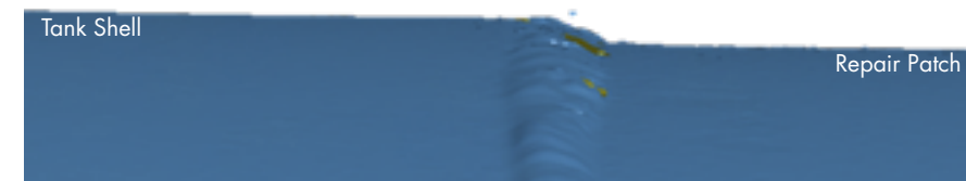
FIGURE 3. Deviation Analysis (Leak Location)
