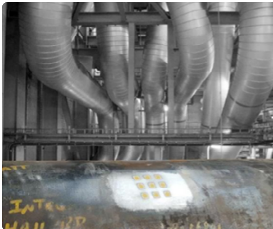
FIGURE 1. Photograph of an ultrasonic thick-film array for monitoring wall-thickness over a critical area of a component.
