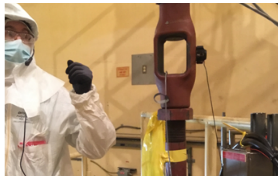
FIGURE 2. Lift rig turnbuckle outfitted with AE sensor.
