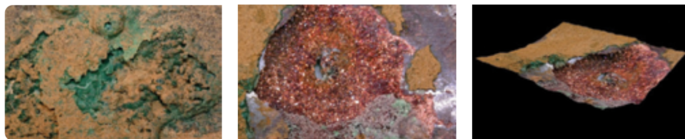
FIGURE 3. Two- and three-dimensional images of a copper heat exchanger tube that has been damaged from under-deposit corrosion (UDC). The image at left shows the typical appearance of the ID deposits. The center image shows a region of damage surrounding a pinhole leak. The 3D image provides an idea of the depth of internal corrosion in the tube.
