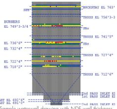
Sample waterwall drawing with NDE wall thickness readings
