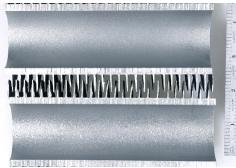
Deposit loading coupons before and after cleaning from tube with light deposits.
