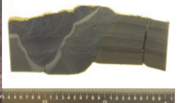
Failed downstream Weld/Elbow
