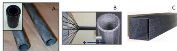
Fig. 1. Examples of SiC and SiC Composite Components: (A) Ceramic Tubular Products triplex LWR cladding, (B) A version of the General Atomics LWR cladding, and (C) A BWR SiC/SiC channel box fabricated and tested by EPRI. (Adapted from Reference [6]).
