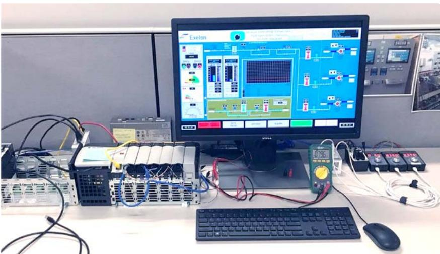
FIGURE 5. Limerick Unit 2 HWC Control Desktop Simulator System
