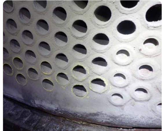
(b) Tube-to-tube sheet joint leak at location of high stresses predicted by FEA
