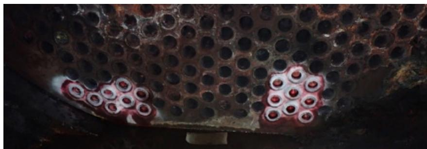
(a) Plugged tube-to-tube joints
