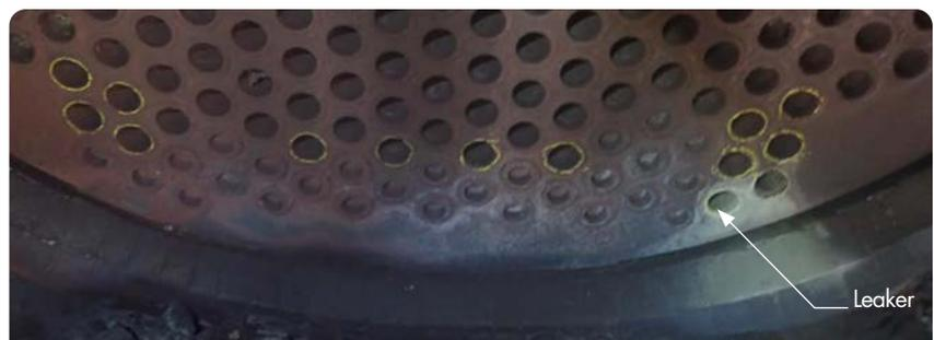
(b) Tube-to-tube sheet joint leak at location of high stresses predicted by FEA
