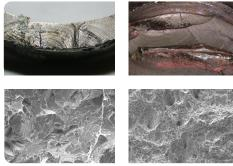
TOP LEFT Beach marks on a fatigue fracture surface TOP RIGHT Keyence image showing fatigue fracture origin area BOTTOM LEFT SEM image showing cleavage (brittle) fracture BOTTOM RIGHT SEM image showing dimpled (ductile) fracture component
