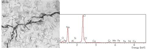
Chloride stress corrosion cracking in an austenitic stainless steel and EDS analysis results from crack deposits showing a very high chlorine peak
