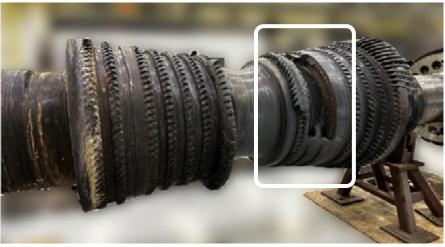
FIGURE 3. IP Rotor Shaft Denoting Area of Liberated Material
