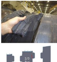
FIGURE 4. Primary Fracture Location
