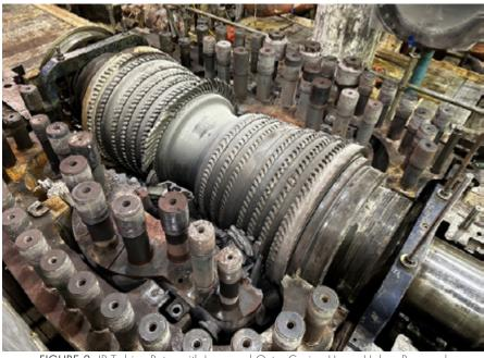
FIGURE 2. IP Turbine Rotor with Inner and Outer Casing Upper Halves Removed
