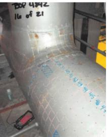
FIGURE 5. Sweepolet Tee with Gridded UT Markings
