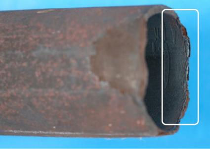
FIGURE 2. Tube to header weld crack.
