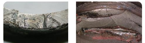
TOP LEFT Beach marks on a fatigue fracture surface
