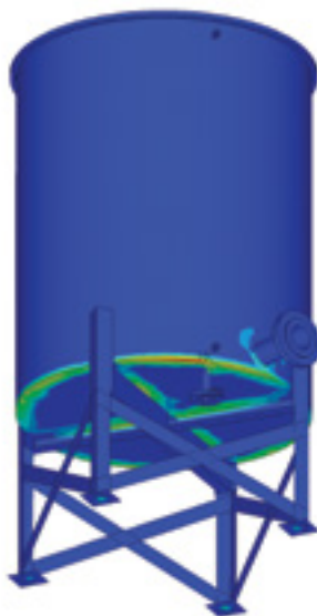
Figure 3. Results of final load combination series with all loads superimposed. Principal stress contours, controlling load combination
