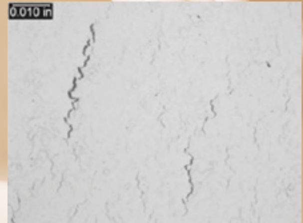
Figure 3. Grain Boundary Graphitization within the Base Metal (Bend Region, Unetched, Transverse Orientation)
