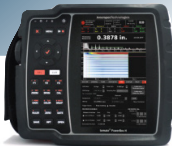
Figure 4 The temate® PowerBox H ultrasonic pulser (top) and an assortment of EMAT sensors and dry- and air-coupled sensors (bottom).
