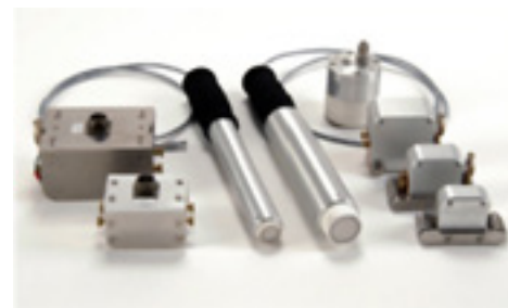
Figure 4 The temate® PowerBox H ultrasonic pulser (top) and an assortment of EMAT sensors and dry- and air-coupled sensors (bottom).
