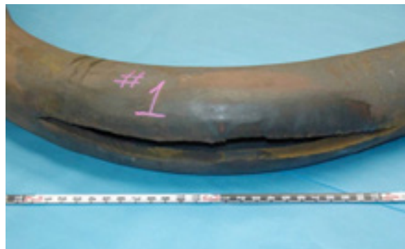
Figure 1. View of the Thick-Lipped Extrados Rupture
