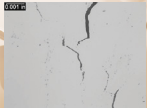
Figure 4. Same as Figure 2, Higher Magnification View of Graphite Along Grain Boundaries
