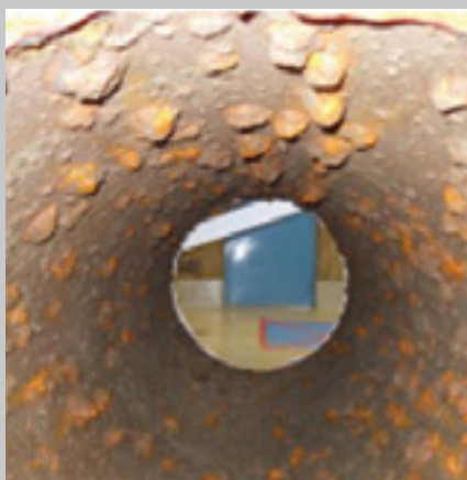
Figure 3. (Left) Internal build-up on a section of piping replaced. (Right) Close-up of an internal pit.
