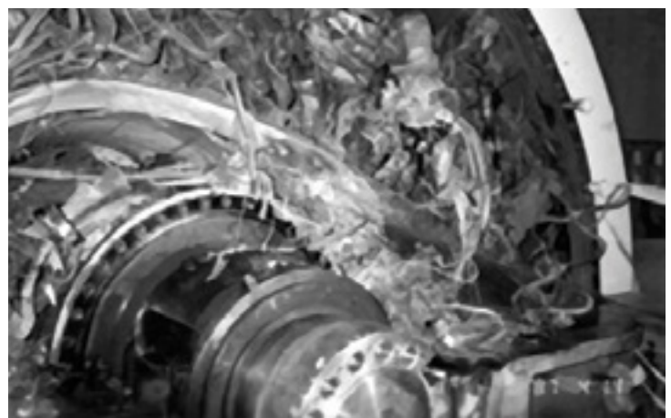
Figure 1. Catastrophic failure of Retaining Ring
