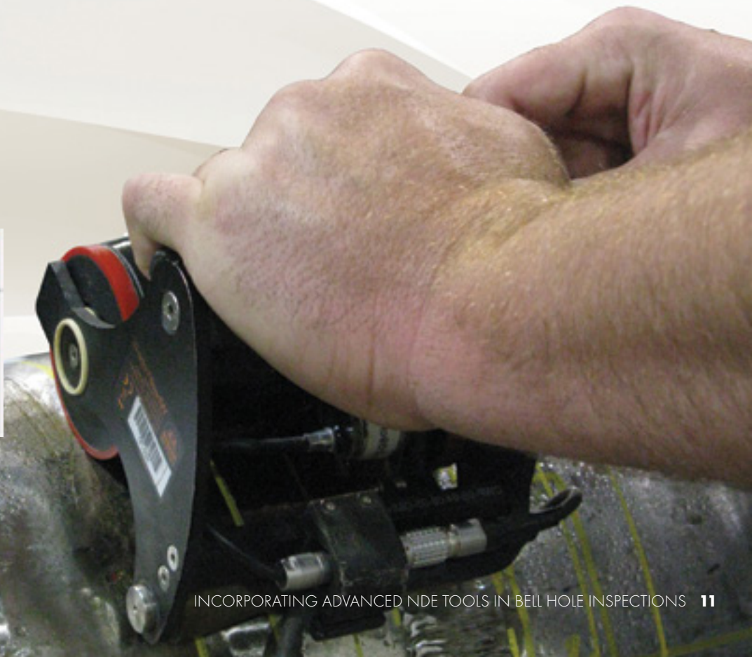
Figure 2: Illustration of the Roller Probe and Scanned Output of Corroded Area
