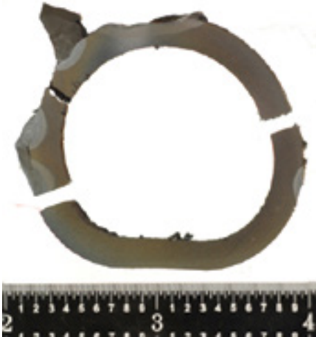
Figure 1. Corrosion fatigue cracking between a membrane and a cold side attachment.
