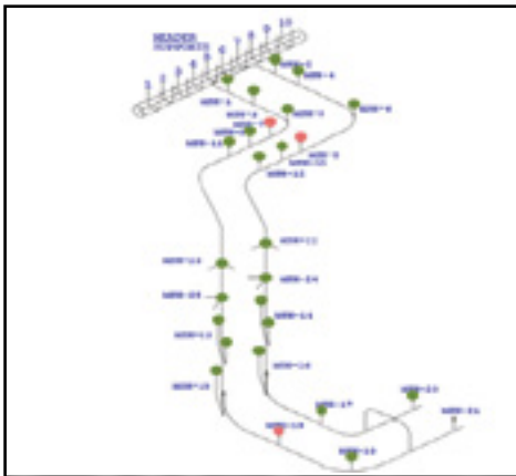
Example displaying hanger inspection results
