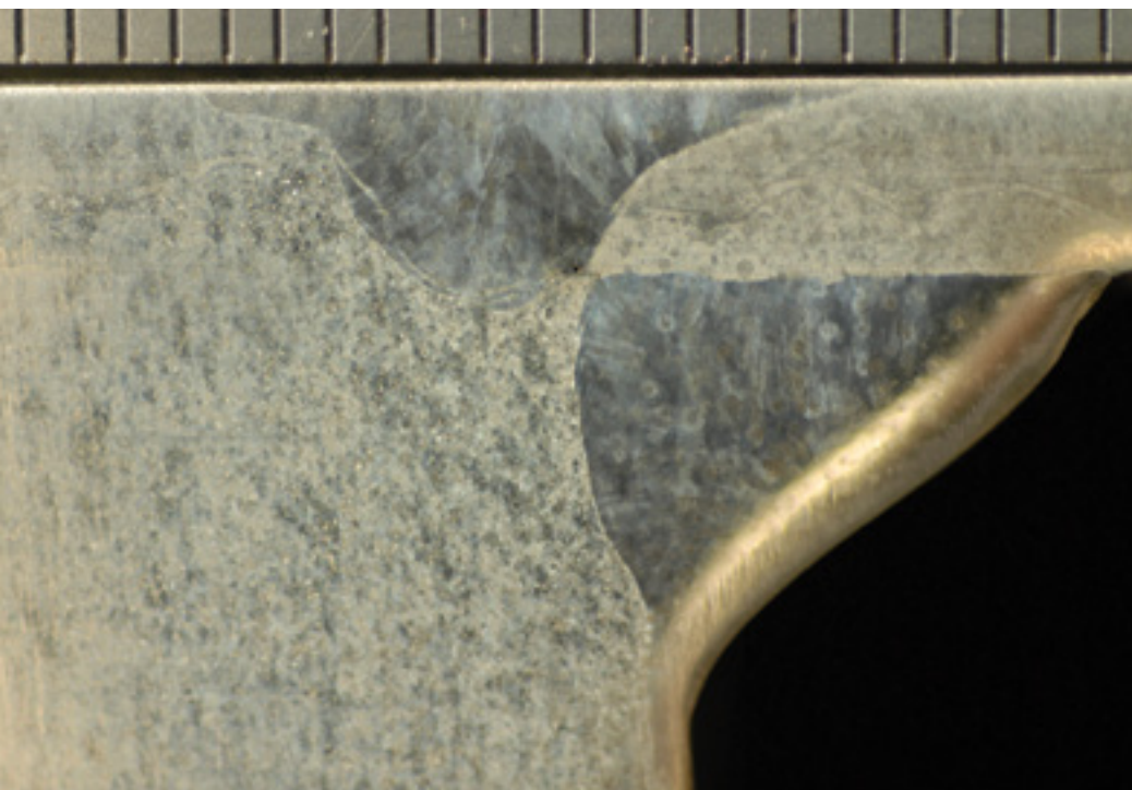
Figure 1. Macrograph of Phased Array UT Development Sample Representative of Typical Joint Configuration (mm scale)
