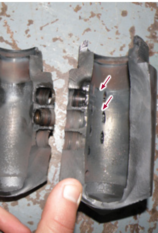
Photo 2: Cracks initiated on ID of attemperator nozzle at "church window" cutouts for orifices. Crack through entire assembly on face containing the section views of orifices. Cracks initiated at red arrows.
