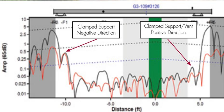
**Figure 2.** Conventional guided wave inspection results of a clamped support pipeline section.
