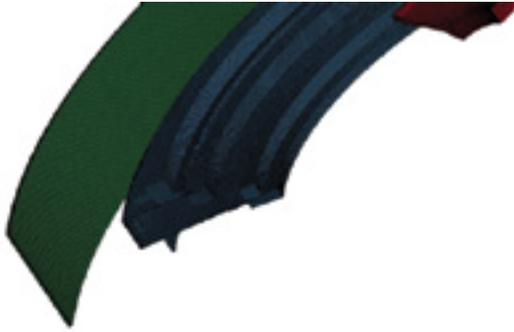
**Figure 2.** Finite element mesh showing mesh resolution and geometric detail of the stationary targets.
