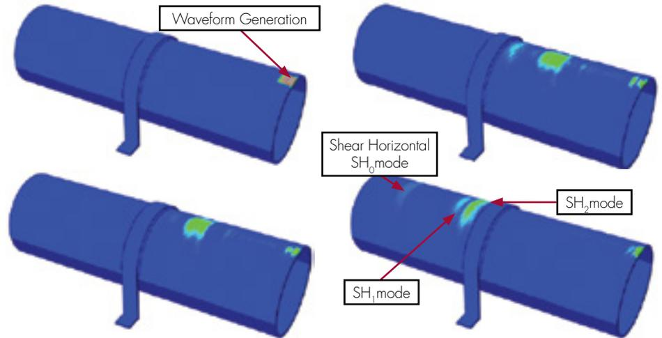
and the presence of a reflection from the support in the positive direction is questionable, the SR-GWT data is consistent. The SR-GWT data consistently produced no reflection from the clamps and is thus not convoluting any potential corrosion indications.
