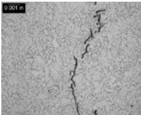
**Figure 4.** Higher magnification views of shock wave damage cracks reveal the step-wise secondary cleavage cracks that are indicative of shock wave cracking.
