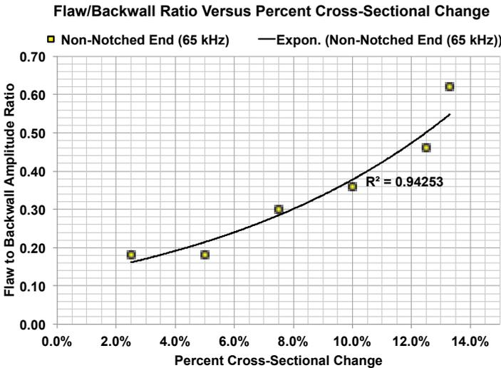
**Figure 8.** Experimental results from the flaw sensitivity study showing the amplitude ratio of the flaw/cut-end echo as a function of percent cross-sectional area of the flaw.
