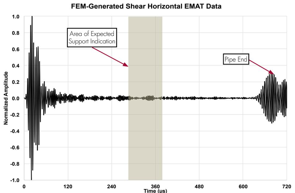
**Figure 6.** FEM generated waveform showing a pulse-echo shear horizontal guided wave.
