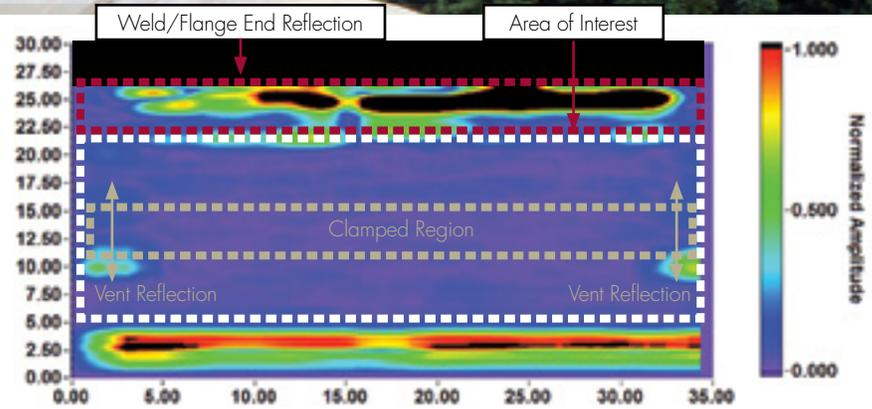
**Figure 4.** Inspection results using our SR-GWT technique on the clamped support in the negative direction located adjacent to a flanged end.
