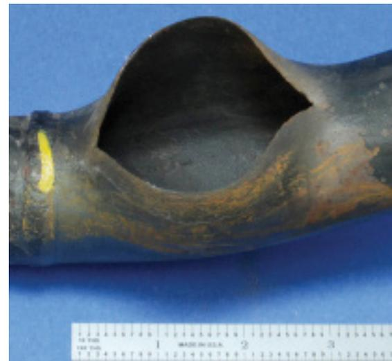
A thin-lipped, fish-mouth rupture in a T91 final superheater tube
