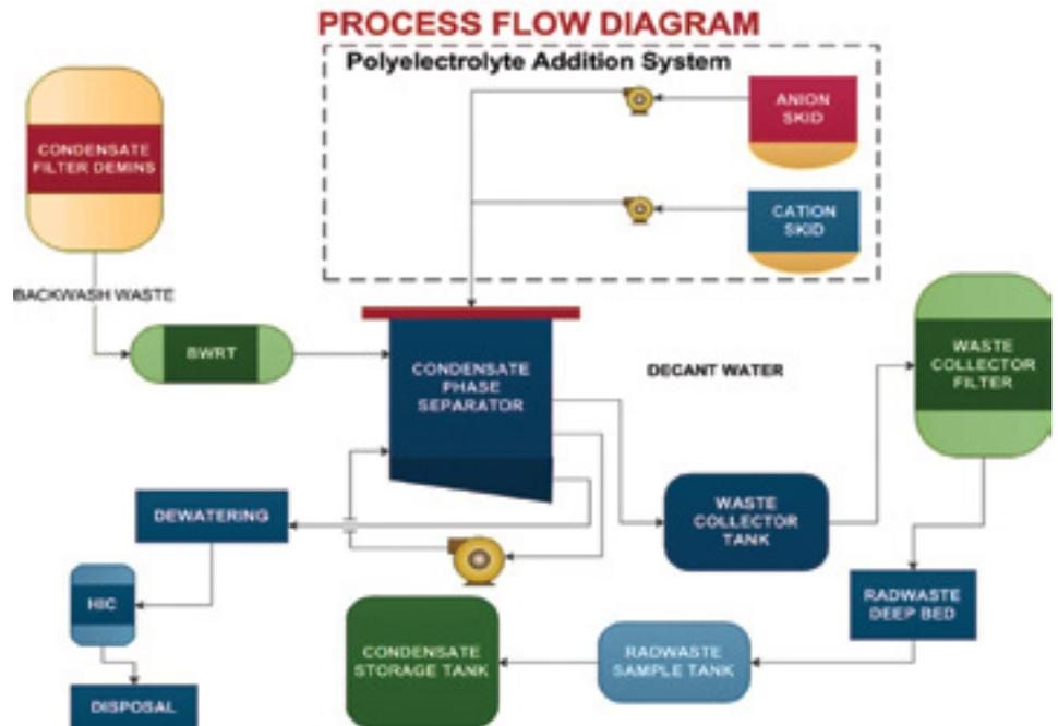
Figure 1. Condensate Filter Backwash Process Flow Diagram
