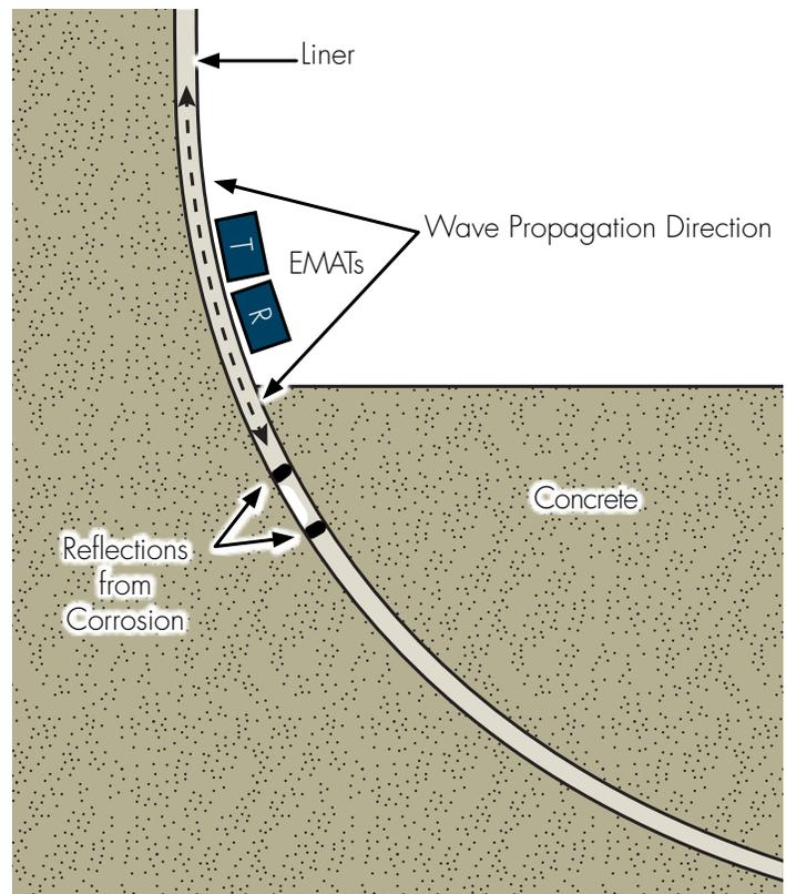
**Figure 1:** Conceptual illustration of EMAT guided wave inspection concept for containment vessels and liners.
