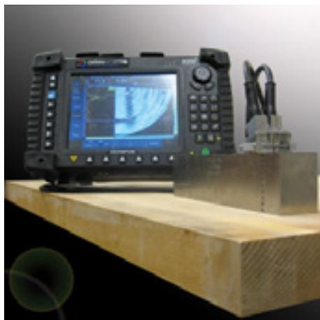
performed to detect indications parallel to the weld and perpendicular to the weld (e.g., transverse cracking). To achieve this, the weld must be inspected from four directions which occasionally require that the component surfaces be contoured to support the probe orientations. Any indications found are evaluated based on permissible lengths and the amplitude of the UT signal as compared to the calibration holes or notches.
