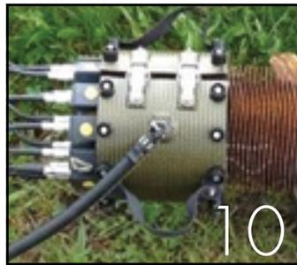
**10 Rapid, Non-Invasive Screening of Finned Tubes with Guided Wave Testing** ■
