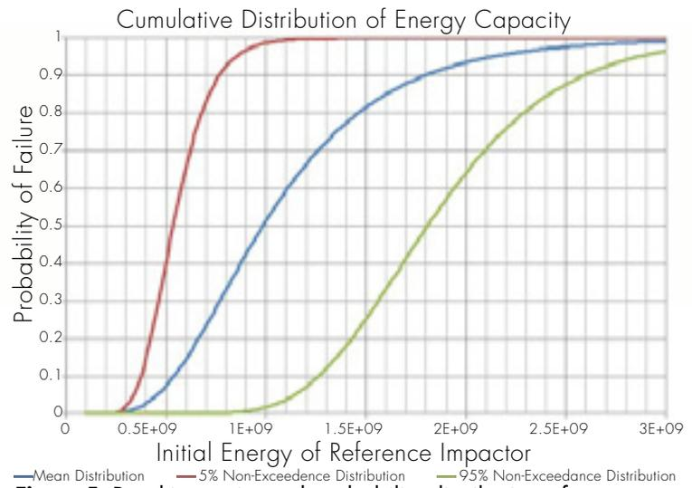
**Figure 5.** Resulting estimated probability distribution of energy capacity (ejection fragility curve) for the illustrative case.
