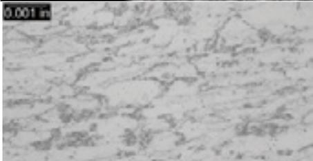
Cross-section from the T91 tube rupture, showing significant grain elongation and microstructural degradation (top image)
