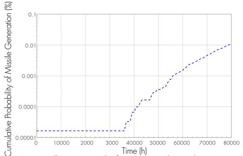
**Figure 6.** Illustrative result of analysis producing the time-dependent turbine missile generation probability,  $P_1$ .
