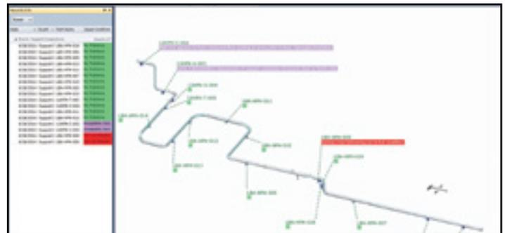
**Figure 5. Pipe Support Inspection Findings**
