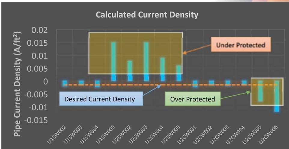
with insufficient CP polarization (i.e. under-protected). These segments require additional anodes, rearrangement of proposed ground beds, or increased output from existing ground beds to mitigate the threat of external corrosion. Similarly, The bars highlighted in the lower half of
