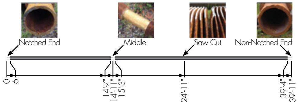
**Figure 6.** Schematic of the experimental flaw detection test setup.
