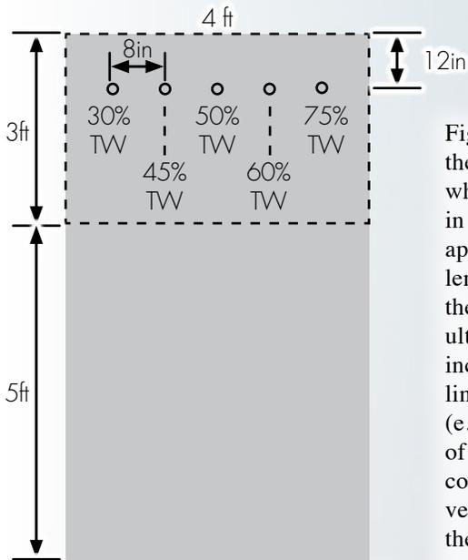
**Figure 2:** Illustration of containment liner mock-up used for testing SR-GWT EMAT technique.
