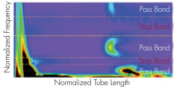
**Figure 4.** Frequency sweep results from the finned tube.
