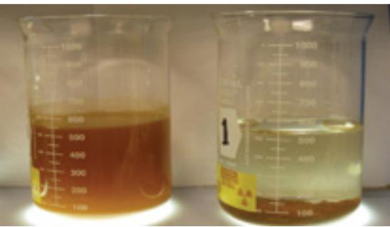
**Figure 2.** Jar Test Results: Left (before) and Right (after) polyelectrolyte addition.
