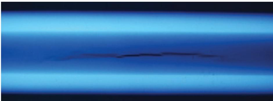
**Figure 5.** Radiographic image of shock wave damage in a superheater tube.
