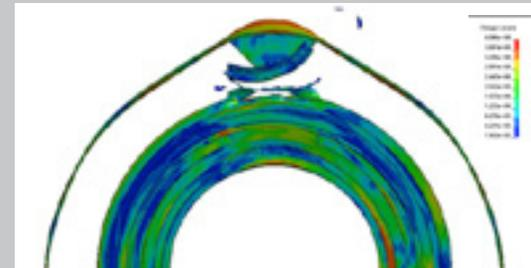
**Figure 4.** Containment of disk fragment as realized from LS-DYNA analysis for bounding case 2.
