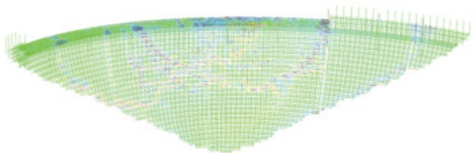
Axial Strain in Reinforcement Layer Added As Part of Retrofit Design
