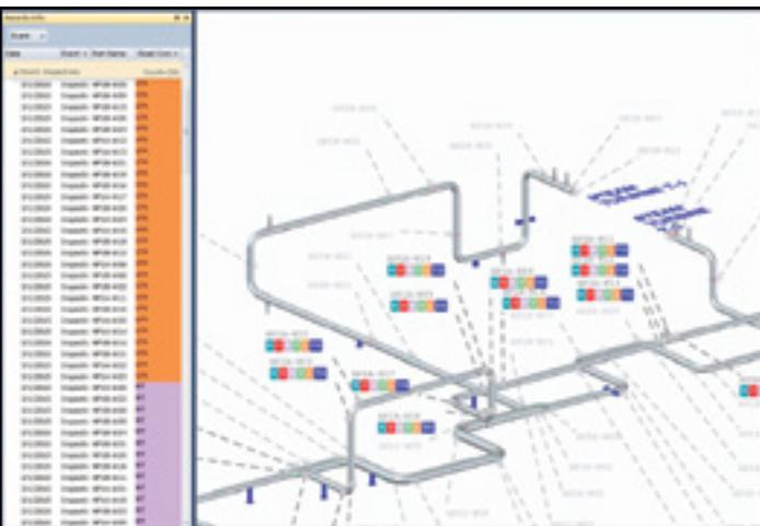
**Figure 4. Graphical Display of Planned Inspection Techniques**
