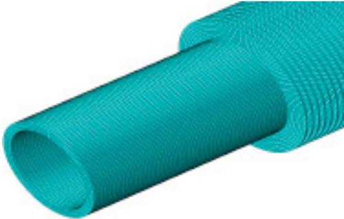
**Figure 2.** Zoomed image of the finite element mesh.
