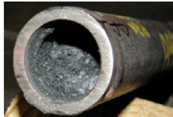
Exfoliated oxide in a finishing superheater tube
