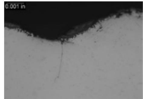
Stress Corrosion Crack
