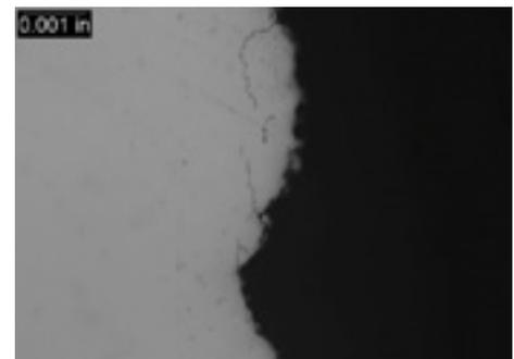
Stress Corrosion Crack
