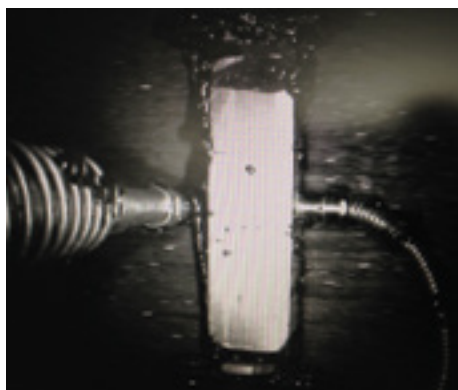
Figure 1. Still frame from onboard camera video feed showing the SIPEC sensor scanning through significant sludge accumulation.
