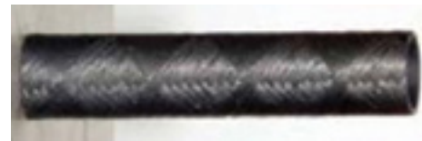
Figure 4. Proposed prototype SiC composite cladding tube sample
