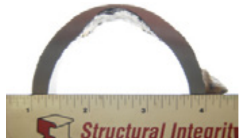
Cross-section through gouge on ID surface
