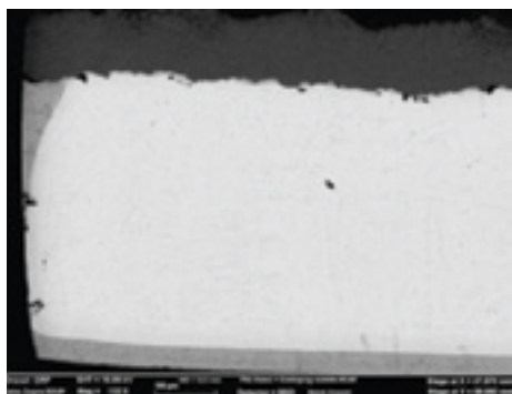
Figure 3. Cross section of a Ti2AlC coated Zircaloy coupon after steam oxidation under LOCA conditions
