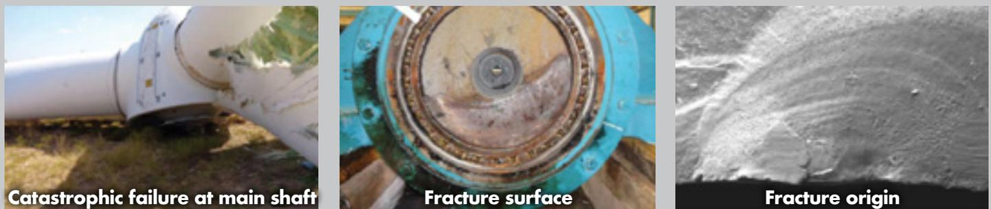
**Figure 2.** Macro and microscopic inspection of main shaft
