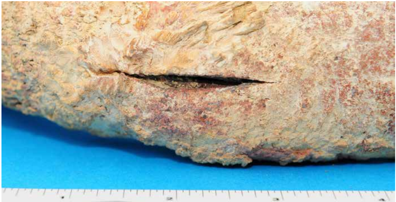
Thick-edged longitudinal rupture in tube section
