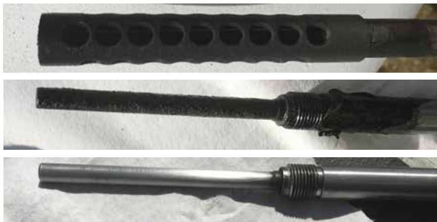
FIGURE 4. TOP ER Probe as removed MIDDLE ER Probe with Velocity shield removed BOTTOM ER Probe after samples collected &amp; cleaning
