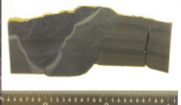
Failed downstream Weld/Elbow
