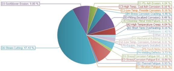
Typical pie chart for various types of failure mechanisms
