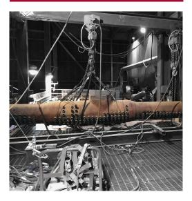
In conventional coal and gas fired fossil plants, boilers are the most likely source of a forced outage due to the wide array of damage mechanisms affecting tubes, headers and piping. Because of this, we have well-defined techniques to optimize reliability through condition assessment and lifecycle management of various boiler components.
