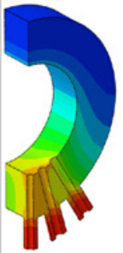
Temperature gradients in outlet header
