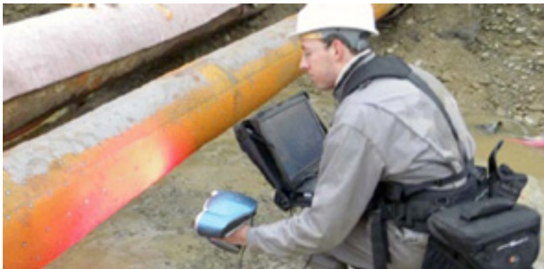
Figure 9: Handyscan 3D laser scanner.
