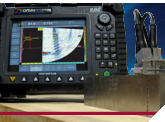
Figure 3: Linear Phased Array (LPA) ultrasonic S-scan image of a series of side drilled holes down a calibration block with angle sweep of 30^\circ to 85^\circ .
