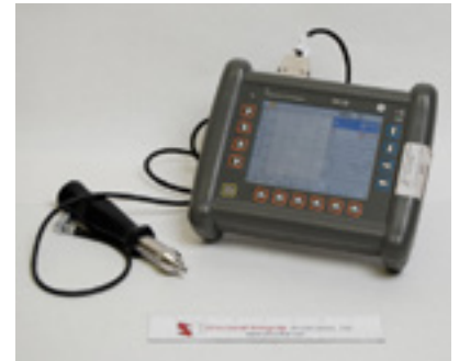
Figure 13: UCI MIC 20 harness tester.
