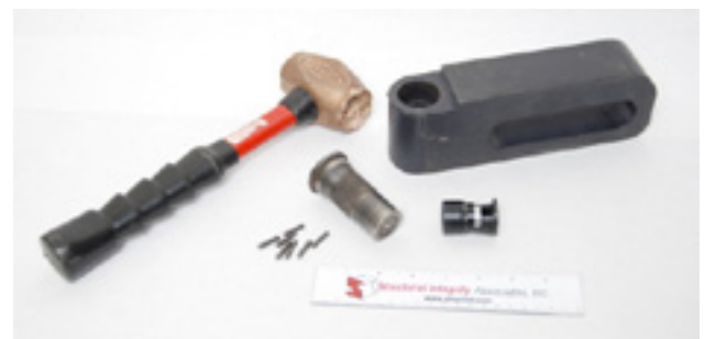
Figure 14: Brinell Method harness testing equipment.
