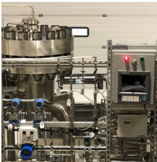
To meet criteria for intergranular stress corrosion cracking (IGSCC) mitigation and inspection relief for vessel internals and piping, BWRs using noble metals + hydrogen need a method to accurately inject a catalyst into the feedwater over long periods of time. A passive platinum injection system is needed to perform this function while meeting the intent of Delivering the Nuclear Promise®.
