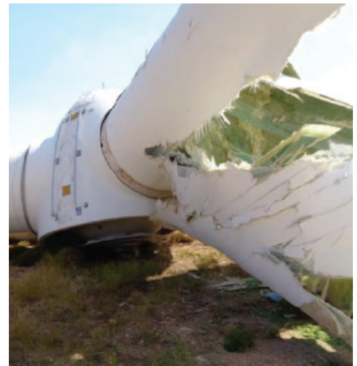
Catastrophic failure at main shaft
