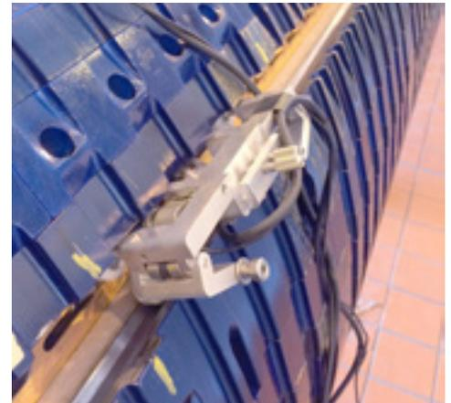
Generator rotor dovetail inspection
