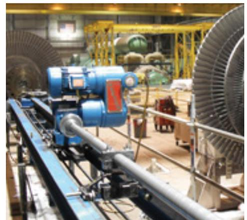
Rotor bore machining and surface conditioning
